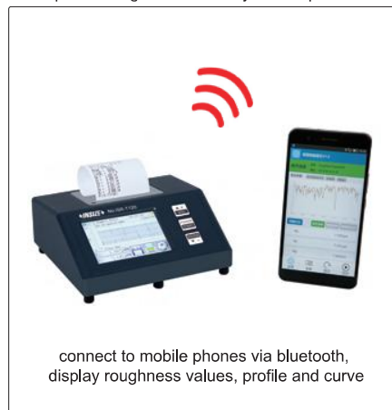
operate roughness tester by mobile phones
