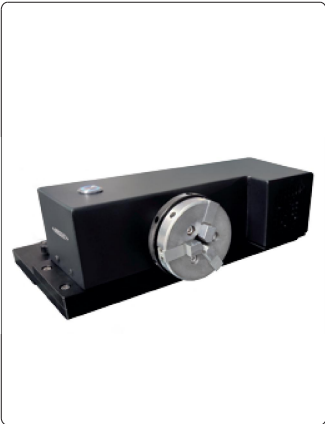
rotary table (optional), maximum clamping diameter 60mm, rotation angle resolution 0.02°, rotation range 360°, rotation speed 12~120RPM
